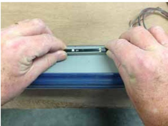
15. Insert circuit board into IAVC1 (Input).
